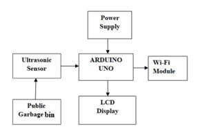
Fig.1 Block diagram
